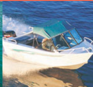
3. 4-5mm plate alloy hull for added strength
