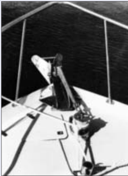
Foredeck arrangement is excellent - with custom made ground tackle fabrications more than adequate for the displacement of this cruiser.
