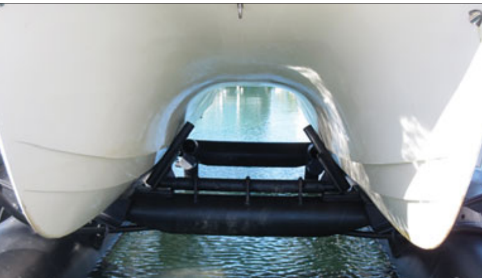
Above: From the water this is what you have got to aim at. Tolerances driving a catamaran are much tighter than with a mono-hull. Twin motors mounted wide are an assistance but approach to an Airberth in a cat are far from lassaize faire . Below: This picture is complementary to that of the Airberth ready to receive a vessel. As the knuckle of the bows come onto the forward crossbeam, small ramps (not seen) provide for a smooth arrival on top of the crossbeam and the angle guides do the job for lateral centring. It is still pretty easy, just not as easy as the promo DVD infers.
