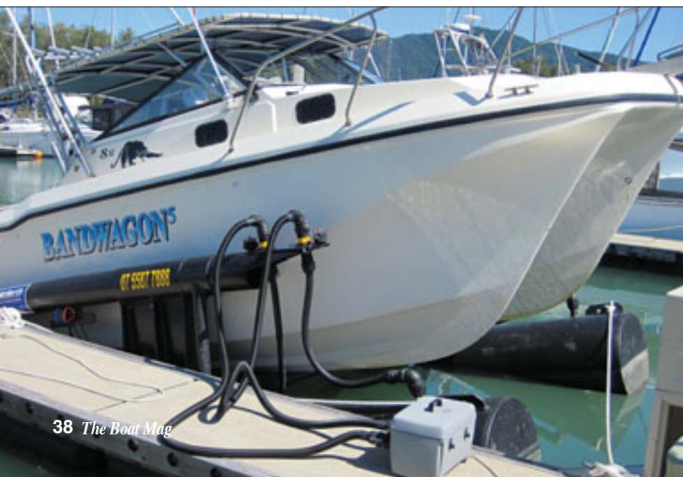
Left: The blower box is pretty easy to handle and it is important to know which switch blows air into the outside pontoon. Air friction means that the outside blower needs to be started first by a few seconds to keep the lift even. When both are running you need to be aft tending the aft mooring rope to make sure the ladder hardware does not snag the marina finger. Once it is all running the process is surprisingly swift.
