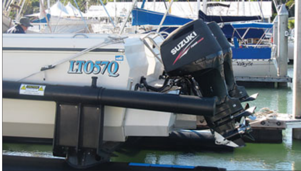
Above: This is about the amount of tilt we leave on the motors for launch and retrieval. The need for it is not too apparent at this stage but if you forget it the consequences of dunking part of the powerhead would be regrettable.
