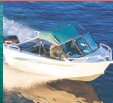
3. 4-5mm plate alloy hull for added strength.
