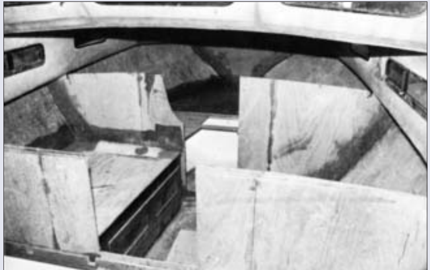
The internal fit-out uses the traditional system bonding a series of ply bulkheads into the hull between the inter-connected glassed in "furniture". A very strong, but time consuming building procedure.
