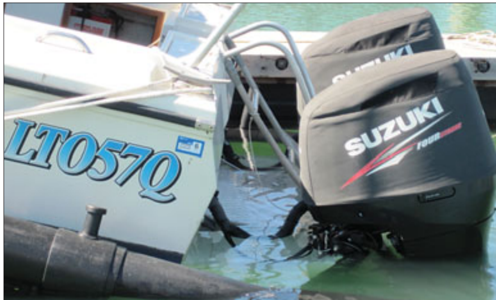
Below: What goes down at the back must come up at the front. The forward mooring rope can go to the outside pontoon and thus needs no adjustment but hull and motor access at the back means that the aft rope goes to the dockside pontoon and thus must be adjusted in use.
