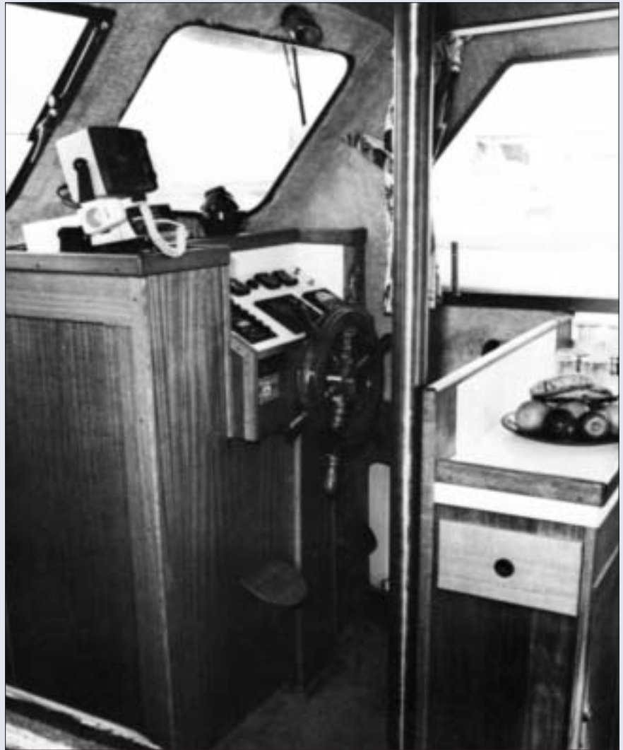
Lower helmsman's station is both comfortable and practical. Observe the Tasmanian oak joinery - a nice change from teak. Where does he sit? Answer: that white flap on the galley folds down on two supports (out of sight) to form a comfortable perch.
