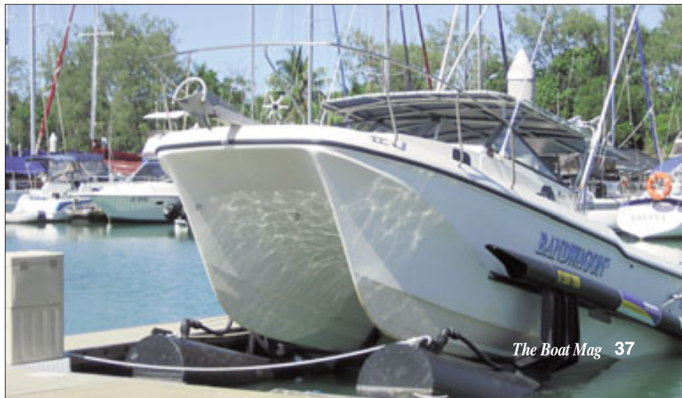
Below: What goes down at the back must come up at the front. The forward mooring rope can go to the outside pontoon and thus needs no adjustment but hull and motor access at the back means that the aft rope goes to the dockside pontoon and thus must be adjusted in use.
