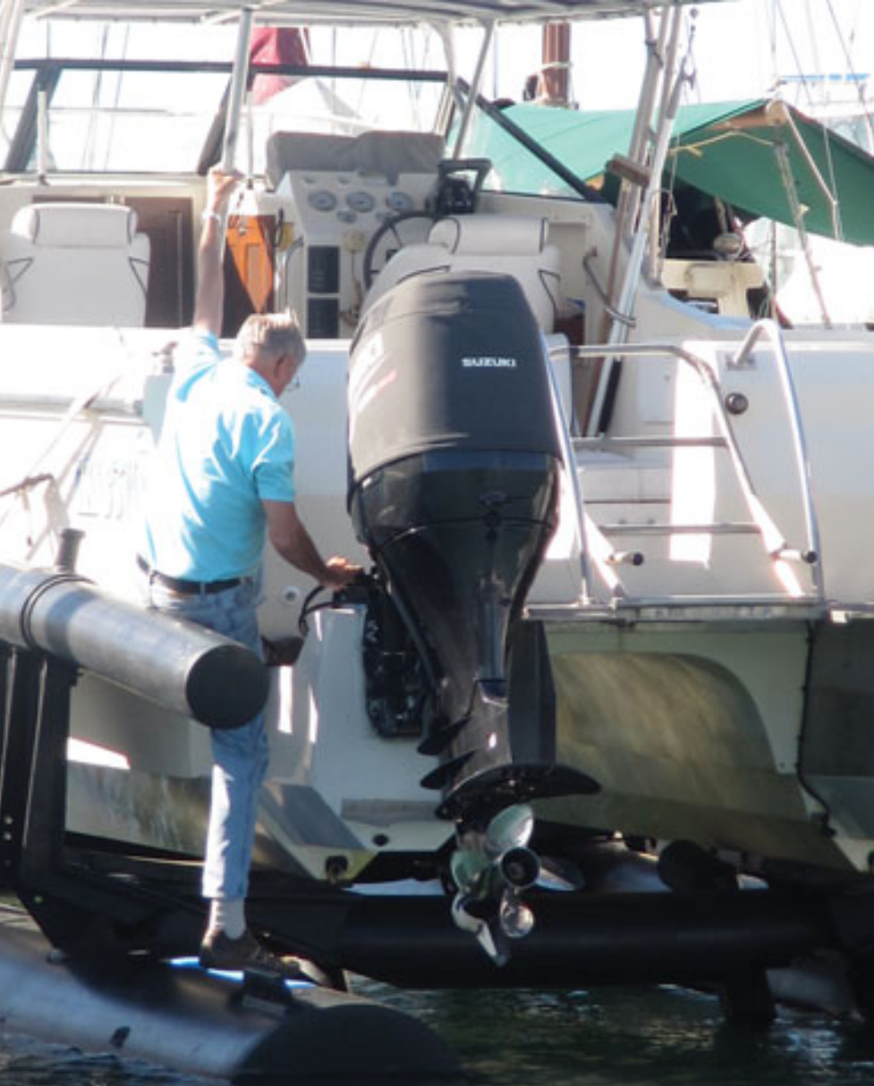
Even for an old bloke like me, with appropriate anti-slip protection, access to the pontoons for drains, motor flushing etc is quite reasonable. It is all a lot easier if you have a good hand-hold, as I have here with an aluminium tube in the aft rod holders.
