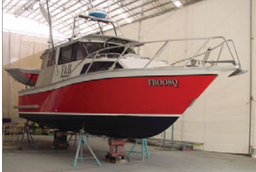
This is a lovely hull shape, with a finish closer to GRP than most alloy boats. The surface coating is 2-pack urethane from PRO-TEC finishes, originally applied by Pat Davey in Cairns. Several years later, it still buffs up beautifully. The anti-fouling (International's Interspeed 2000) has coped well with being taking in and out of the water, too.
