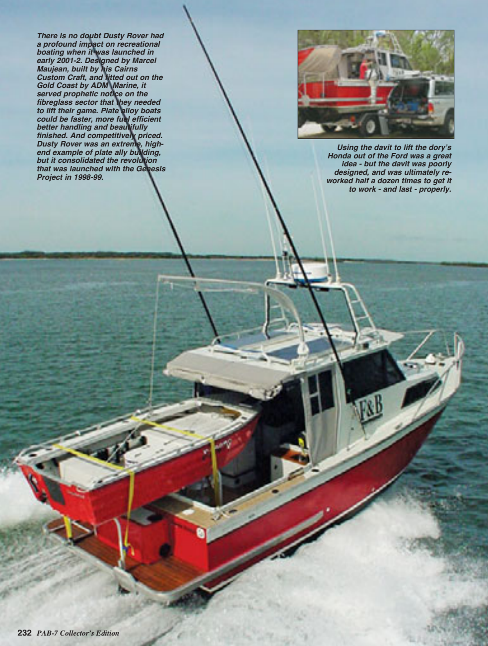
This is a lovely hull shape, with a finish closer to GRP than most alloy boats. The surface coating is 2-pack urethane from PRO-TEC finishes, originally applied by Pat Davey in Cairns. Several years later, it still buffs up beautifully. The anti-fouling (International's Interspeed 2000) has coped well with being taking in and out of the water, too.
