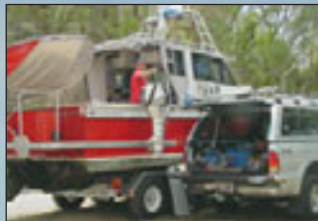
Using the davit to lift the dory's Honda out of the Ford was a great idea - but the davit was poorly designed, and was ultimately re-worked half a dozen times to get it to work - and last - properly.
