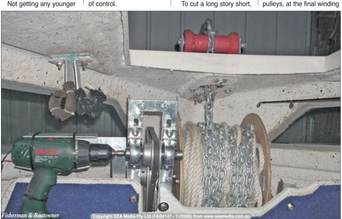
radius of about 150mm, approx 225Kg pulling power is generated. (When most of the rope is out, the pulling power is many times that).
