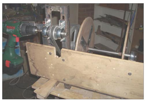
about 80rpm at the winch with the belt reduction. A belt drive was chosen because it is very cheap, keeps the drill away from wet areas and I can easily change ratios if necessary.
